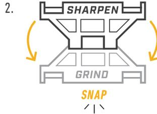
Flip Edge Guide down and out of the way to make belt changes easier. Snap into place.
