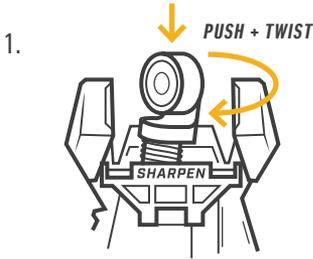
Push tensioner down and rotate clockwise  $\frac{1}{4}$  turn to lock in place.
