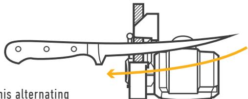
**TIP:** It may be necessary to repeat this alternating process of bevel sharpening and back honing to achieve the sharpest results (no burr).
