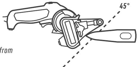
\* Pull up on the Angle Guide to remove from the Sharpening Cassette.
