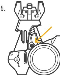
The belt tracking screw (on back of sharpener, with guide removed) can be adjusted to correct belt tracking.
