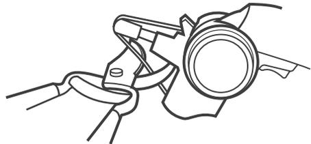
\* Pull up on the Angle Guide to remove from the Sharpening Cassette.
