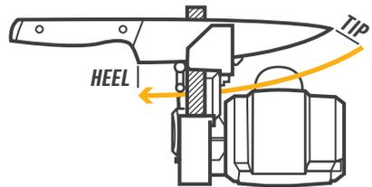
**PROPER TECHNIQUE:** Keep the blade in the slot, up against the amber line on the Angle Guide and with the blade resting on the Edge Guide. Maintain this position and stop as the tip reaches the center of the belt.
