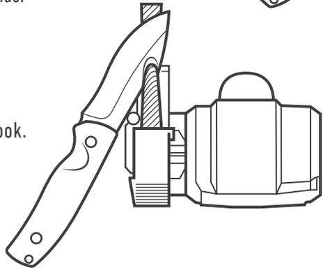
\* Pull up on the Angle Guide to remove from the Sharpening Cassette.
