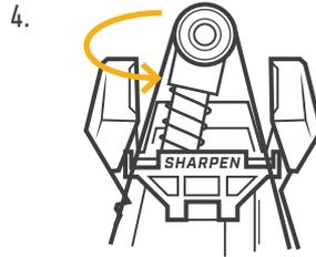
Turn tensioner  $\frac{1}{4}$  turn counter-clockwise to release. Spin belt by hand to ensure properly centered on pulleys before powering up. Return the Edge Guide to the up position.
