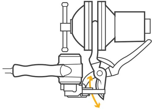
**NOTE:** Some tools require the anvil to be inserted through the grinding frame opening (as shown) to allow belt access to the cutting edge.
